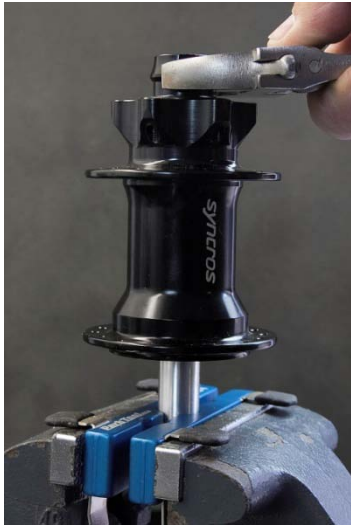
FIG. 6 These photos show the correct use of the Park Tool Axle Vise to remove axle end caps. This tool, or a tool like it, is essential to service the hubs correctly. Make sure to use the center clamp for the inner axles when removing the end
